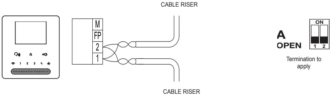
Connecting the indoor station art. 7539 in the terminal configuration (REF. SI696).
