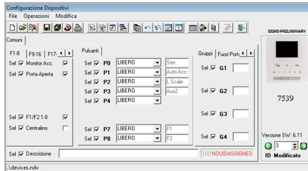
It is possible to change button configurations, create groups, select chime tune types, adjust chime volume and enable or disable functions. On completing the desired settings:
