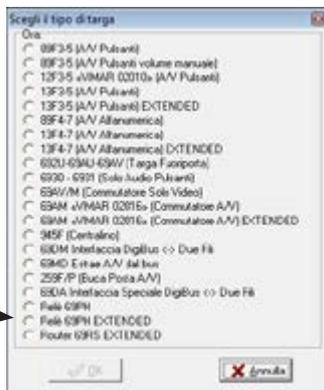
Select the icon highlighted by the arrow in Figure 6, the window appears where you can select the Relay 69PH EXTENDED). After confirming with OK the configuration window will open for the 69PH.
