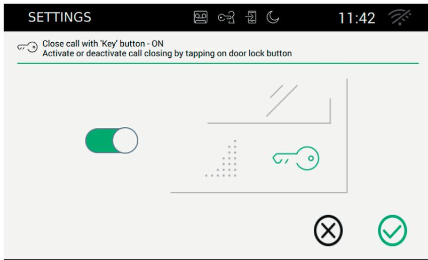
Operate the sliding button to enable the function.
