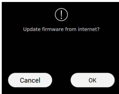
This operation could take a few minutes. On completion of the updating procedure, the device will restart automatically.
