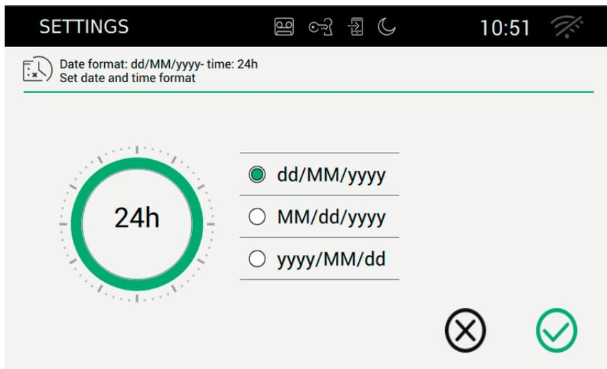
Set the time format to either 12 h (am-pm) or 24 h by pressing the corresponding button
