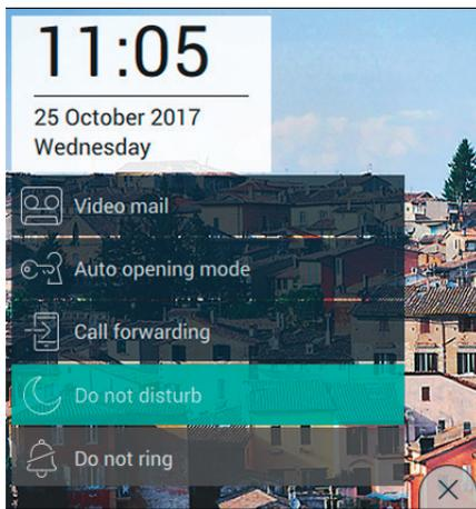
While the Do Not Disturb function is activated, it is not possible for the user to activate the Do Not Ring function.
