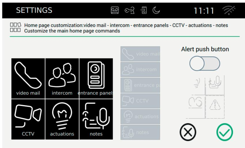
Drag the function, while holding it pressed, into the desired square. The selected destination square will turn green; Release the function to confirm its position.
