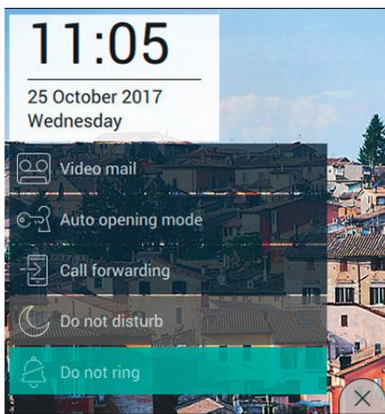
While the Do Not Ring function is activated, it is not possible for the user to activate the Do Not Disturb function.
