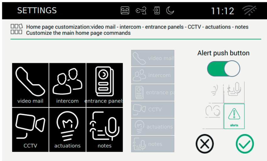
When the Alarm button is enabled, the appearance of the Home page is as shown in the image below:
