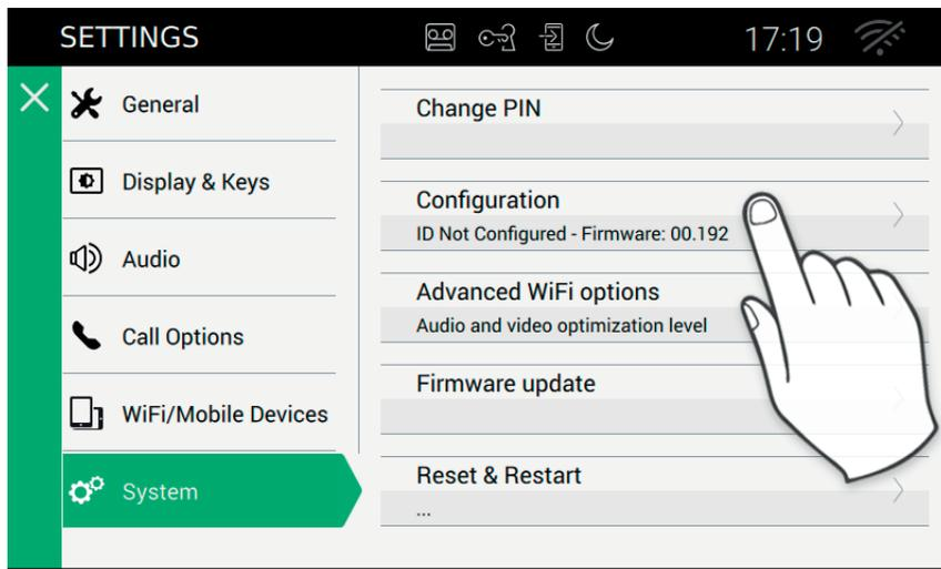
Before the device is put into operation, it must be assigned a unique ID in the 2-wire bus system.
