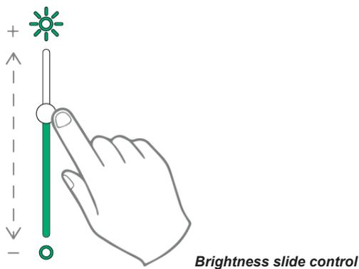
The brightness and volume controls described above only have effect during calls. The levels are not saved in the settings of the 7" EVO video entryphone.
