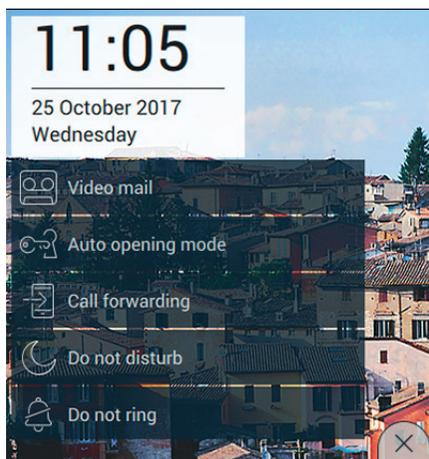
The quick commands remain available for 30 seconds, after which the application will return to the normal display mode. If you want to close the menu sooner, simply press the close tab (
