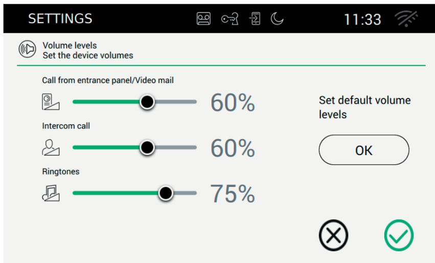
To set the desired levels, move the corresponding sliders to find the optimum volume.
