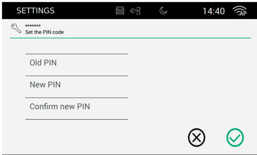
To change the PIN, first enter the old PIN and then the new PIN. Confirm the new PIN to ensure that you have not entered the wrong PIN by mistake.
