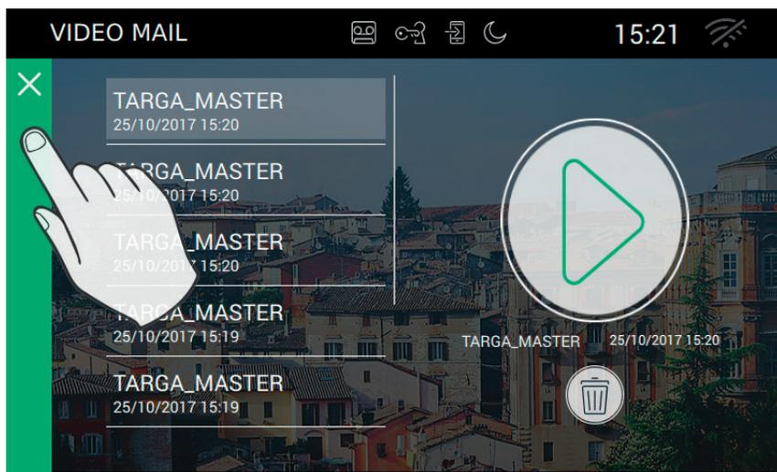
The page presents the messages in chronological order, with the last message to be recorded at the top of the list. Each call or videocall is identified by the name of the device from which the call was made, plus the date and time at which the recording started.
