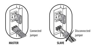
When a call is received, the MASTER video handset of the system rings and switches on, while the video handsets configured as SLAVE only rings.
