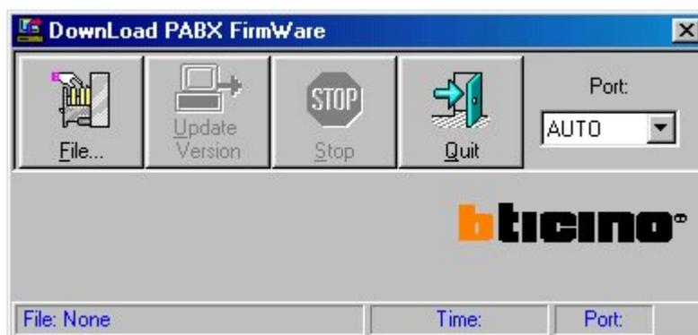
To send new firmware version to the telephone exchange, it is possible to select serial port that the device is connected or to select Auto option that the software scan all system serial port to find the telephone exchange.
